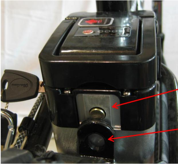
This hardened steel safety bolt is shown in place, locking the battery in the guide sleeve
